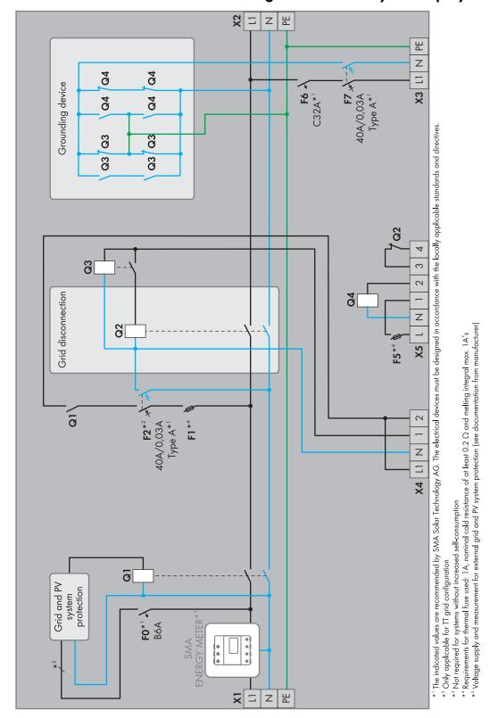
Figure 3: Schematic diagram of the automatic transfer switch for a single-phase battery-backup system in Great Britain/Northern Ireland
