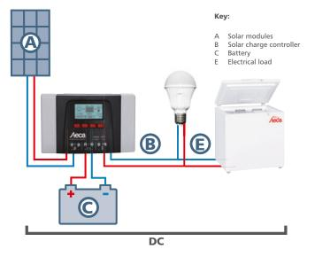
**Generator function:** Using the generator function, the Steca Tarom – based on the SOC or the battery voltage – can start a generator automatically when the battery is discharged and switch this off again when the battery is full. Using the surplus manager, an additional load can be activated automatically when the battery is full. This is switched off again as soon as no more energy surplus is available in the solar system. This guarantees that all available energy is used.
