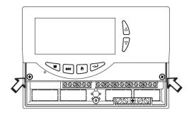
Remove with the help of a tool the plastic from the openings provided for the cables pass-through.
