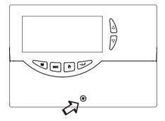
Remove the two screws shown in the drawing, then remove the whole body from the base.
